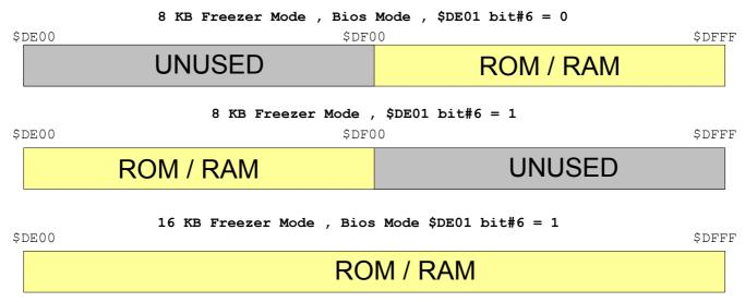
To add Action Replay compatibility, which has only 8KB of RAM, an additional bit was introduced in the Retro Replay to allow banking in the I/O area. Setting bit#1 of \$DE01 allows all banking bits to be enabled in the I/O area, disabling this bit disables banking bits 13-15 in this area. When in MMC Replay Bios mode, disabling this bit additionally disables banking bits 18-16 in the I/O area.
